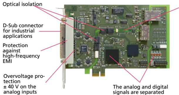
customer requirements. However, it is also ensured that the ADDI-DATA products themselves do not emit high levels of EMC radiation into their surroundings. The function of external devices in the immediate surroundings could be heavily affected by this. This could have particularly serious consequences for medical technology.
